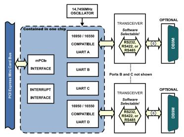
PCI Express Mini Card (mPCIe), a low-profile small-footprint bus standard originally intended for adding peripherals to notebook computers, has become the de-facto standard for highperformance, small form-factor devices in many applications.
