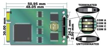
Configuring a port's Termination switch in the Terminated position applies a  $120\Omega$  load in series with a  $0.01\mu F$  capacitor across the Rx+/Rx- pair in RS422 mode, or across TRx+/TRx- in RS485 mode.
